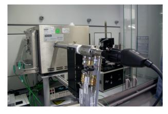
The temperature on the back of a coated steel plate (75 mm x 75 mm) is recorded during the test to evaluate the performance of the coating. The specimen is positioned vertically in the door of the furnace. The method produces representative residues that can be used for advanced analysis after testing. The STT MuFu<sup>+</sup> generates reliable, repeatable results on fire resistance on the small scale.
