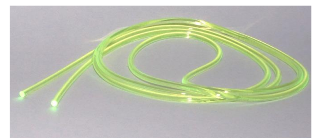
Fig. 2. green fluorescent silicone step-index E-POF with an outer diameter of 2 mm
