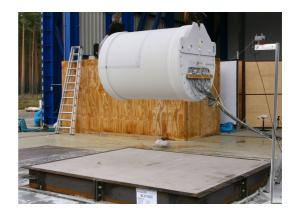
Storage containers for radioactive waste with negligible heat generation for the Konrad repository have to withstand drop tests without impact limiters onto a concrete plate of a specified strength class. The left figure shows the stress distribution in a cylindrical cast iron cask at the time of maximum load during a 0.8 m drop, calculated by using FEM. The lid is blanked for a better visualization. Numerical analyses have the following functions in such scenarios:
