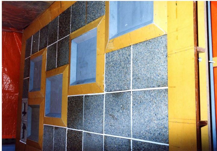
Figure: Vertical wall with concrete samples and steel moulds for testing concrete protecting products with special testing regulations.
