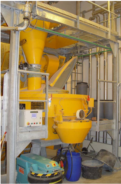
View at the mixing installation with right: 250-l-mixer and left: 500-l-mixer, vacuum cleaner, scales and silo-installation
