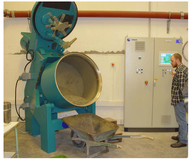
150-l-high performance mixer with control and measuring installation for power, temperature and recipe-management
