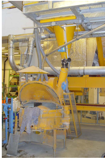
View at the mixing installation with right: 250-l-mixer and left: 500-l-mixer, vacuum cleaner, scales and silo-installation
