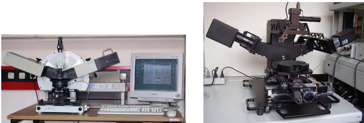
Fig. 2: left: Single wavelength ellipsometer (Sentech SE400) right: UV-vis-NIR spectral ellipsometer (Woollam M2000DI)
