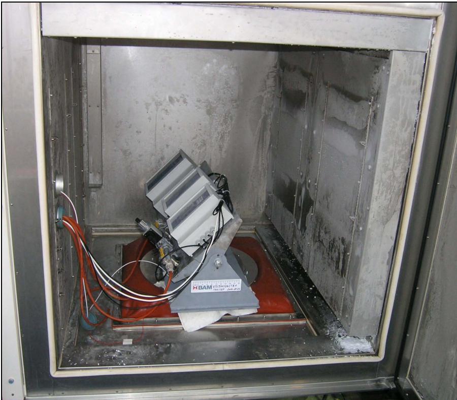
Fig. 1: Climatic chamber with test sample at -18 °C
