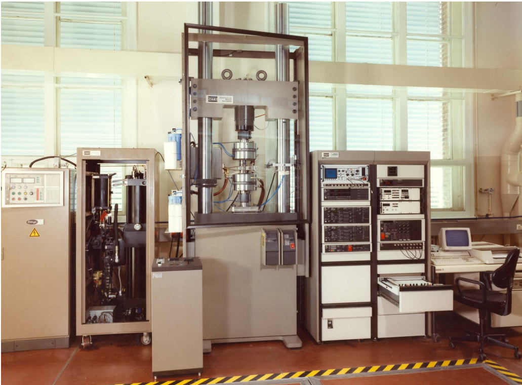
Figure 1: Overview over the test system for axial, torsional and internal pressure loading
