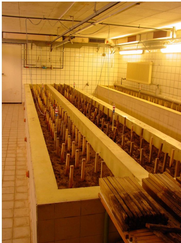
Fig. 1: BAM Fungus Cellar. Tests of wood preservatives for wood to be used in ground contact.
