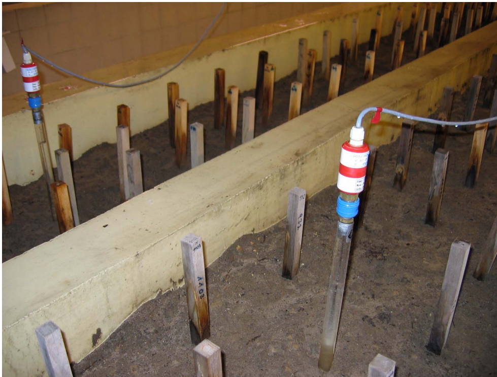
Fig. 2: BAM Fungus Cellar. Tests of wood preservatives for wood to be used in ground contact. Determination of the soil moisture with tensiometers.
