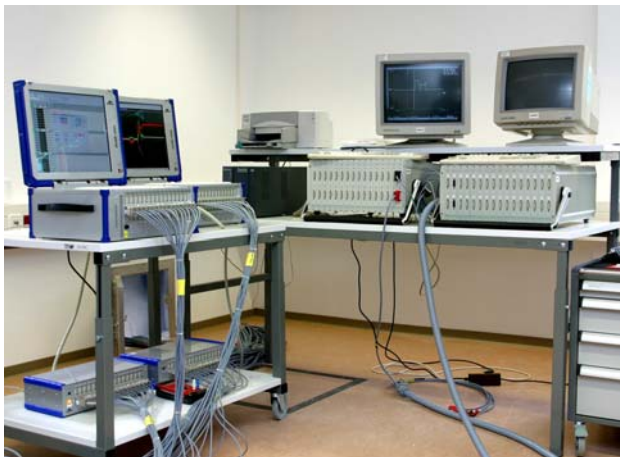
Portable data acquisition systems for dynamic strain and acceleration measurements
