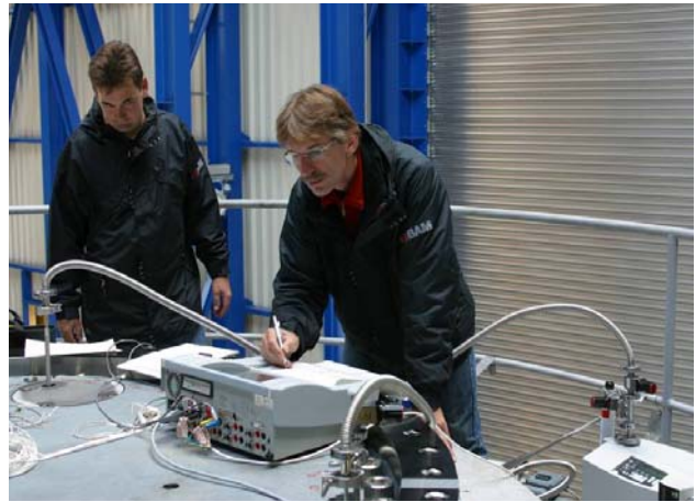
Leakage testing of the closure lid system of a cask
