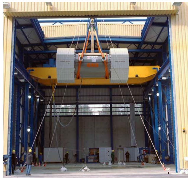
9 meter drop test of a full-scale cask model (181.000 kg)
