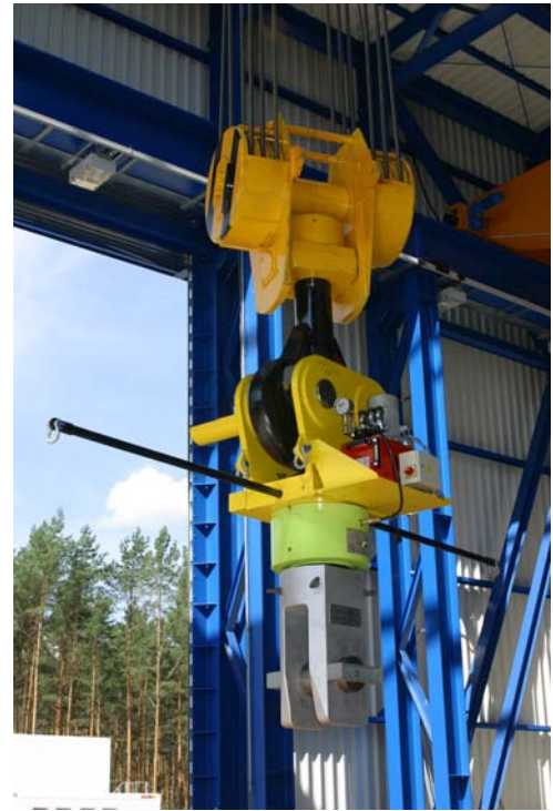
Electro-hydraulic detaching device for test object masses up to 200.000 kg
