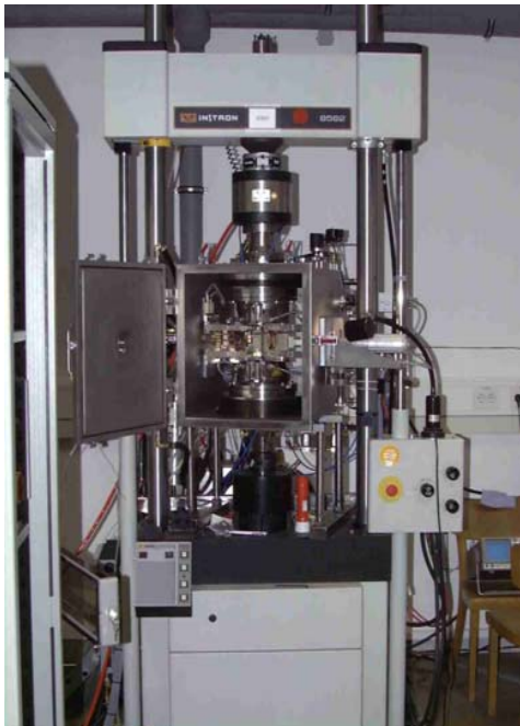
Tensile Testing Facility for Temperatures up to 1900 °C
