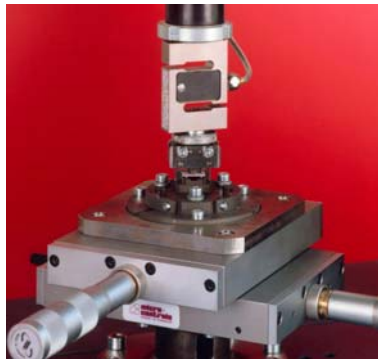
Four-Point bending jig for ceramic laminate and substrates
