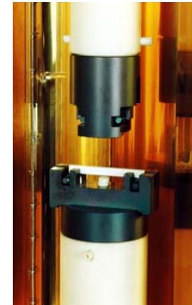
Bending jig located in a furnace
