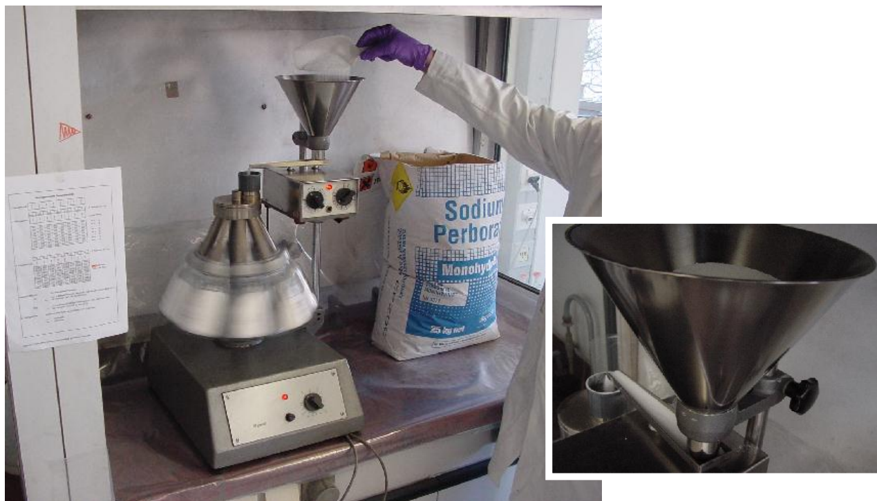
Figure 1: Dividing of the 25 kg sample on a spinning (rotating) riffler at BAM right picture: the sample flows from the hopper to a vibrating chute and travels along the chute to the receivers (8 glass containers)
