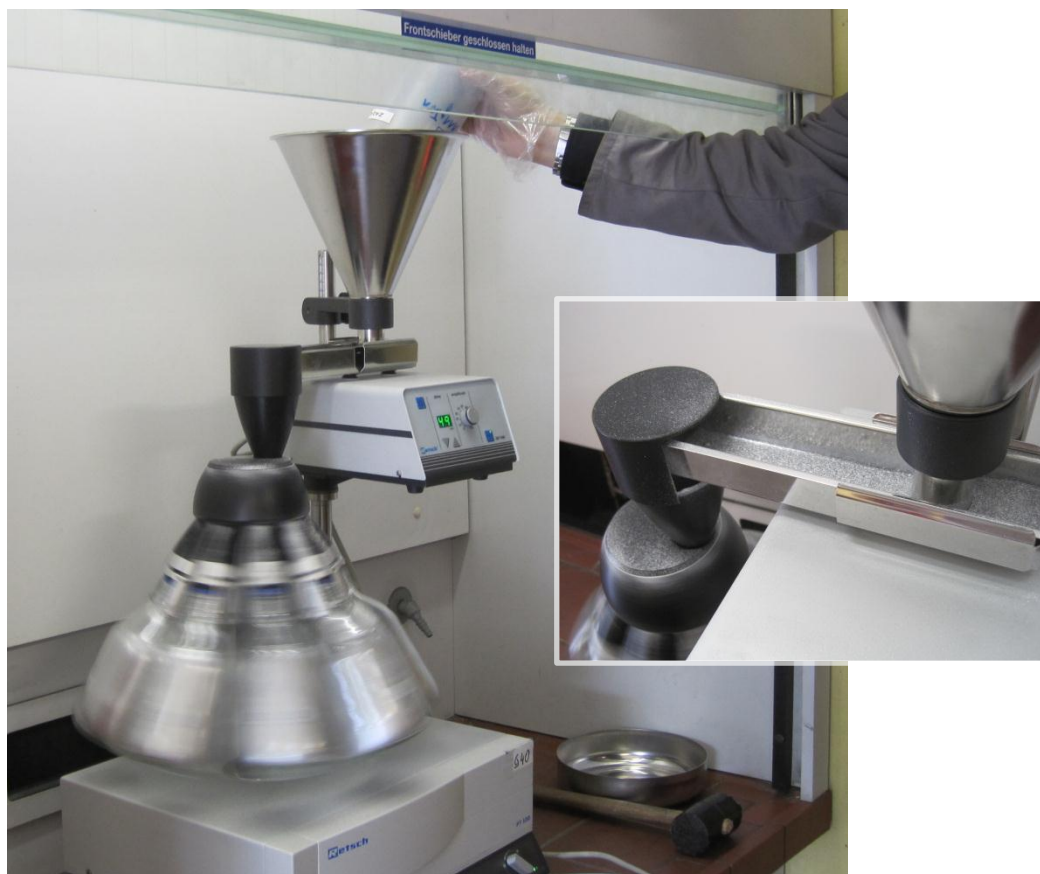
Figure 3-1: Dividing of the 16.6 kg stock sample on a spinning (rotating) riffler at BAM right picture: the sample flows from the hopper to a vibrating chute and travels along the chute to the receivers (8 glass containers)
