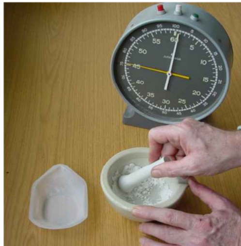
Fig. 1: Mixing by using a ceramic mortar and a pistil instead of a glass beaker and a glass stirring rod
