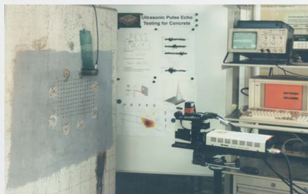
Ultrasonic echo experiment for testing concrete with optical signal detection. A broadband transducer (centre frequency 100 kHz) is in a fixed position and an aperture is scanned using a scanning doppler laservibrometer as ultrasonic signal detector.
