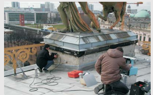
Abb. 4: Radar investigation at the pedestal
