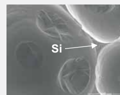
SEM micrograph of nano-composite foam containing 17% silica, detection of SiO 2 particles by EDX
