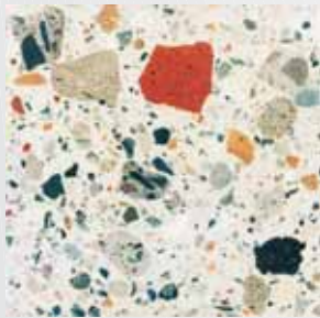
Concrete made with recycling aggregates W
