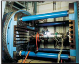
Orbital welding of a supermartensitic stainless steel (SSMS) pipe in the component test facility
