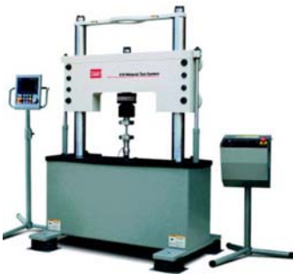
Servohydraulic testing device for superimposed TMF/HCF-loading up to 1000 Hz
